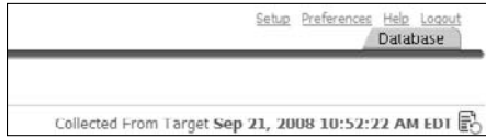
Figure 13-4: The Database tab is at the top right of any page in Database Control.
